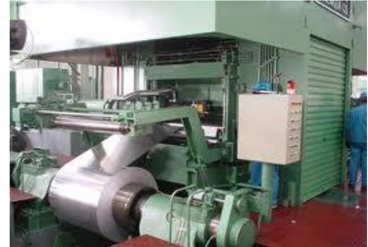
View of Cold Rolling Mill
