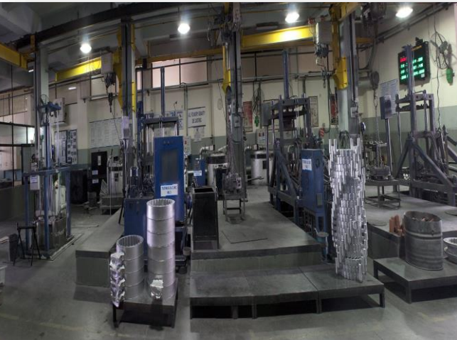
GDC Machines with Tilting capability
