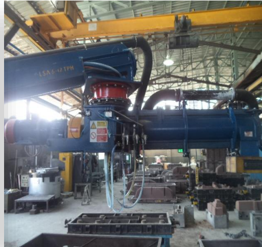
Continuous mixer capacity 12 MT per hour manufactured by Laud's Foundry Eqpt Germany
